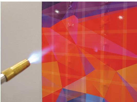
4. Using a foam roller applicator, apply firm pressure over 3-4 rivets at a time. Going over too many rivets at a time may result in tenting because of the film cooling down.
